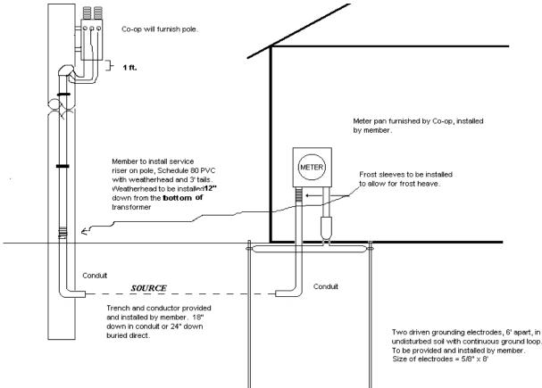
The trench depths specified are minimum and are measured from final grade.
