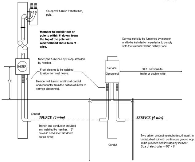
The trench depths specified are minimum and are measured from final grade.
